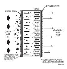
Each time the air circulates through the heating/air conditioning system and air cleaner, more particles are removed. These particles are generated by normal household activities and also enter the house from outside. That is the reason we recommend that you use the air cleaner as much as possible.
