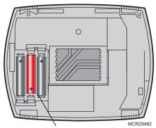
Insert supplied batteries for primary or backup power.
