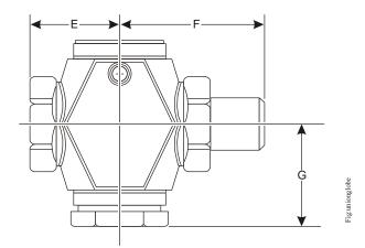
Figure 3: Two-Way N.O./PDTC and Two-Way N.C./PDTO Union Globe Valve Dimensions (See Table 3.)
