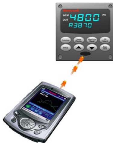
Figure 1-3 Depiction of infrared communications
