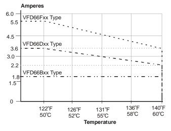
Figure 11: 400/460 VAC Temperature De-Rating
