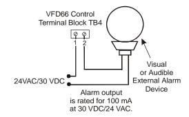
Figure 7: Wiring the Alarm Output
