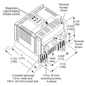
Figure 2: VFD66 NEMA 1 Enclosure Dimensions
