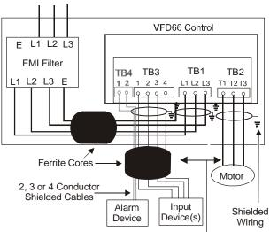
Separate input and output cables. Do not run input cables alongside output cables. Do not bundle input and output cables together.
