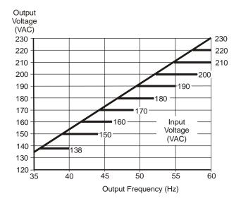
Figure 15: Output Voltage and Frequency vs. Input Power, 208/230 VAC
