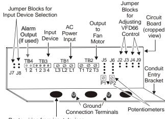
Route wiring from input devices through this conduit entry hole.
