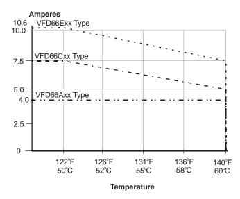
Figure 10: 208/230 VAC Temperature De-Rating
